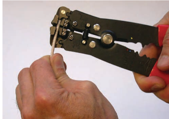
General small gauge wire strippers, hard on XL type wire insulation due to the metal construction.
